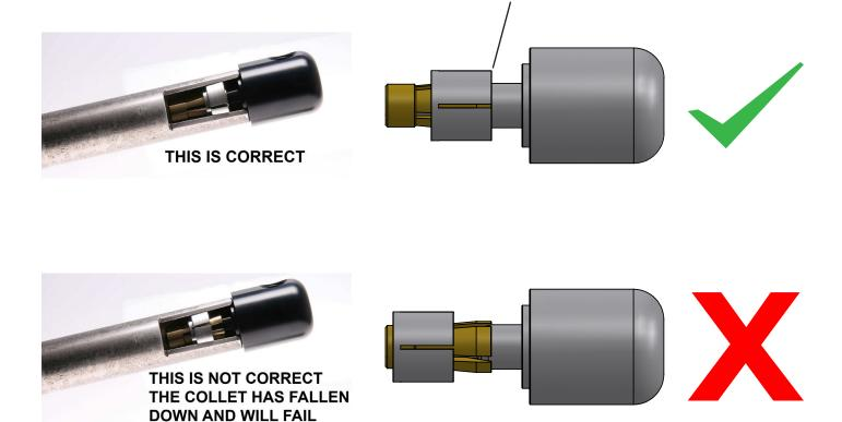
Once your bar end product is installed be sure to regularly and periodically test all fasteners and fittings to avoid product damage. If your product has grub screws, then we recommend using a little thread lock compound for correct fixture. Do not use power tools to tighten the bolts.
